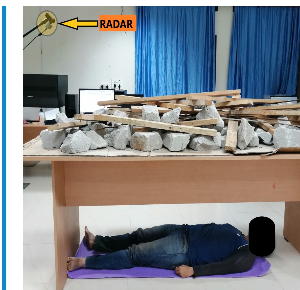
Target lying under a pile of rubble
